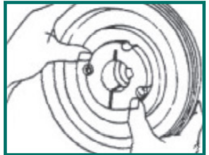
Insert screw and locate on shaft
