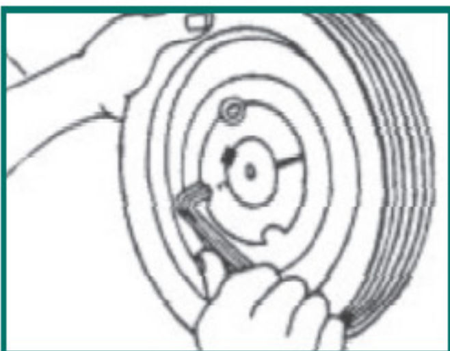
Insert screws in jacking off holes for removal of Taper Bush
