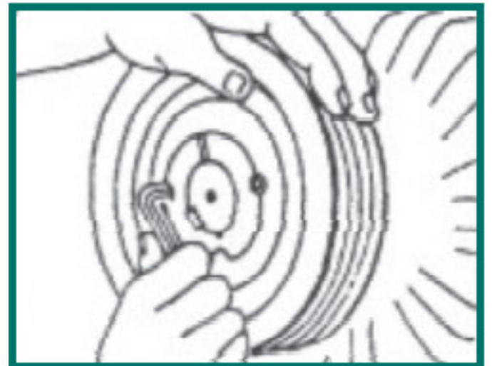
Tighten screws alternately
